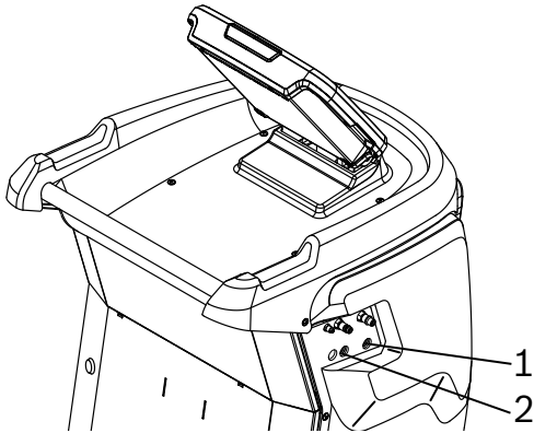
Fig. 12: Service hoses connection (HP and LP)
