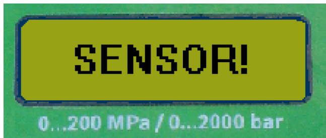
Abb. 12: Failure indication on the digital pressure display unit
